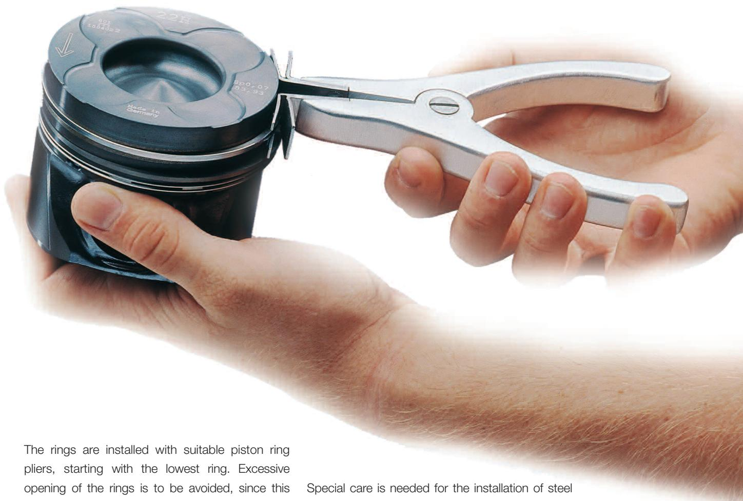
The rings are installed with suitable piston ring pliers, starting with the lowest ring. Excessive opening of the rings is to be avoided, since this could lead to deformation of the rings. If the rings are deformed, they are no longer able to provide a perfect seal. It is of vital importance that the TOP mark be observed. Rings that have the TOP mark are to be fitted with the marking facing upwards towards the piston crown.
