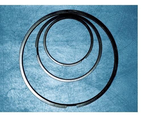
The piston rings are put on with the greatest of care. Each time they are taken off unnecessarily and put back on again with excessive stretching, permanent deformation is caused and the operating performance is impaired.
