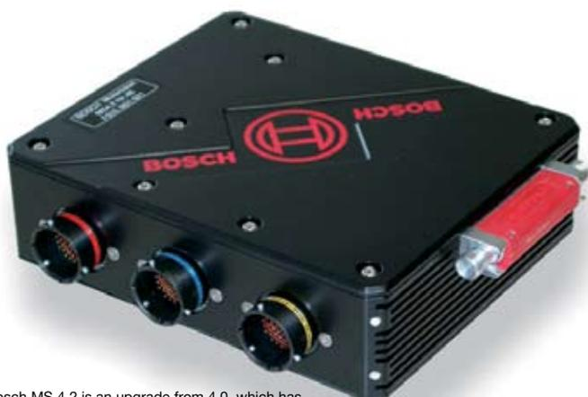
Bosch MS 4.2 is an upgrade from 4.0, which has an additional board and a bespoke housing
