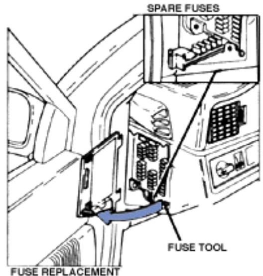
The easiest way to see if a fuse is blown is to remove it. Refer to the list of fuses on the inside of the fuse box cover to see which one should be examined.
