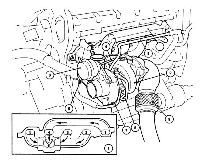
Volvo 850 Turbo (T-5) Exhaust manifold and turbocharger
