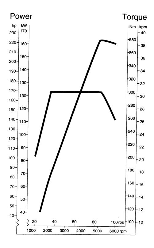
Volvo 850 Turbocharged B5234T engine
